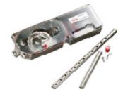
The Intelligent Duct Smoke Detector provides early detection of smoke in the air moving through heating and ventilation (HVAC) ducts in commercial and industrial premises. Its purpose is to prevent the re-circulation of smoke from an area on fire to areas unaffected by the fire when used with a XP95 or Discovery detector.
