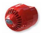
Sonos Pulse conventional wall mounted Sounder Visual Alarm Devices are available with a white and red flash colour. The white flash variant has an EN 54-23 approved coverage pattern of W-3.1-11.3, whereas the red flash variant has a coverage pattern of W-2.4-7.5. The sounder has an a SPL of up to 97dB.
