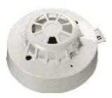
The Discovery UL Heat Detector is distinguishable by the low airflow resistant case and uses a single thermistor to sense the air temperature around the detector.
