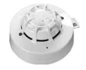
The Discovery Multisensor Detector comprises optical smoke and thermistor temperature sensors which give both a combined signal as well as a separate heat signal for improved false alarm management.
