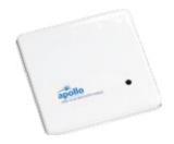
The XP95A 120V AC Input/Output module is a loop-powered device which incorporates a monitored input circuit for connection to dry contacts, as well as a 120V AC 4A rated dry contact relay output. It is mounted in a plastic facia plate for use with a 4[] square or two-gang electrical back box.
