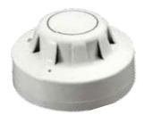
The Series 65 Optical Smoke Detector incorporates a pulsing LED located within the housing of the detector. The external detector moulding is identical to that of the ionisation detector, and has an indicator LED which is clear in quiescent state but produces a red light in alarm.
