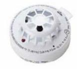
The XP95 I.S. Heat Detector operates by measuring heat levels with a single thermistor which gives an analogue value output proportional to the external air temperature.
