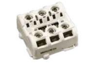
The Mini Monitor Module is an interface within an entirely new housing. This allows the unit to be fitted onto a standard 35mm DIN-Rail (using a twistclick motion) or mounted within an enclosure, for example a pull station. It is designed to monitor the state of one or more single pole, voltage-free contacts connected on a single pair of cables and to report this status to Apollocompatible analogue control equipment.
