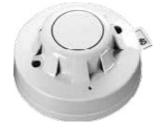
The Discovery Ionisation Smoke Detector uses a low activity radioactive foil to detect fires by irradiating the air in the smoke chambers and causing a current flow. If smoke enters the chamber, the current flow is reduced leading to an alarm.
