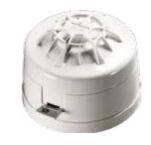
There are two heat detectors in the XPander range, designed to suit a wide variety of operating conditions. A Static Heat Detector (CS) which responds only when a fixed temperature has been reached and a Rate-of-Rise Detector (A1R) which has a fixed upper limit, but in addition, measures the rate of increase in temperature.
