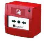
The Discovery Marine Manual Call Point has been approved for use in indoor marine applications. A seven-segment DIL switch enables addressing of each call point at commissioning stage. When operated, the manual call point interrupts the polling cycle for a fast response. Bi-coloured LEDs indicate isolate and normal conditions.
