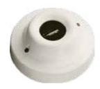
The Marine Series 65 Base Mounted UV Flame Detector is designed to protect enclosed indoor areas where open flaming fires may be expected. The detector has a fast acting response to flames up to 25m away and is equipped with a single UV sensor with a narrow spectral response in order to discriminate between flames and most spurious sources of radiation.
