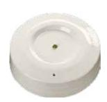
The Discovery Marine Isolator is placed at intervals on the loop and ensures that, in the case of a shortcircuit, only the section between the isolators will be affected. When the short-circuit is removed, the isolators automatically restore power and data to the isolated section.
