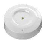
The XP95A Isolator is placed at intervals on the loop and ensures that, in the case of a short-circuit, only the section between the isolators will be affected. When the short-circuit is removed, the isolators automatically restore power and data to the isolated section.
