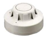
The Series 65A Photoelectric Smoke Detector incorporates a pulsing LED located within the housing of the detector. The detector housing is identical to that of the lonisation Detector apart from an indicator LED which is clear in quiescent state but produces red light in alarm.
