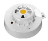
The XP95 Heat Detector monitors temperature by using a single thermistor which provides a count output proportional to the external air temperature. The XP95 range features two heat detectors, standard and high temperature. The standard heat detector is classified as an A2S device and will report an alarm at 55°C. The high temperature detector, classified as a CS device, will report an alarm at 90°C.
