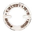
The Series 65A Standard Base has been designed to enable detectors to be fitted without the need of force – particularly useful when fitting to suspended ceilings. All Series 65A bases have a 'one-way-only' fit.
