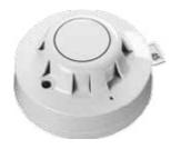
The XP95 Ionisation Smoke Detector uses a low activity radioactive foil to detect fires by irradiating the air in the smoke chambers and causing a current flow. If smoke enters the chamber, the current flow is reduced leading to an alarm.
