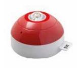
The Loop Powered VAD is designed for indoor use. The Category C VAD is specifically designed for use on a ceiling and comes in two different coverage classes. The two EN 54-23 coverage classes are C-3-8.5 and C-3-15. These devices are used to supplement sounders in areas which carry the risk that sounders will not be heard.
