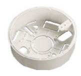
The Conduit Box is a versatile accessory for surface mounting Apollo bases. The box has knockouts to accept PG16 or M20 cable glands, conduit or mini-trunking. Self-tapping screws are included to fit the detector base to the conduit box.
