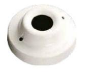
The Marine Intelligent Base Mounted IR<sup>3</sup> Flame Detector is designed to protect all indoor areas, even in dirty or smoky conditions, where open flaming fires may be expected. The detector has three IR sensors that respond to different IR wavelengths to discriminate between flames and spurious sources of radiation.
