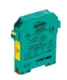
The DIN-Rail Mains Input/ Output Unit provides a voltage-free, single pole changeover relay output and a monitored switch input. The unit supervises one or more normally-open switches connected to a single pair of cables.
