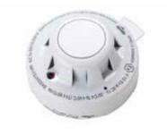
The XP95 I.S. Ionisation Smoke Detector uses a low activity radioactive foil to detect fires by irradiating the air in the smoke chamber and causing a current flow. If smoke enters the chamber, the current flow is reduced leading to an alarm.
