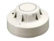
The Series 65A lonisation Smoke Detector uses a low activity radioactive foil to detect fires by irradiating the air in the smoke chamber causing a current flow. If smoke enters the chamber, the current flow is reduced leading to an alarm.
