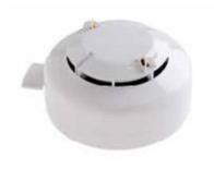
The SOTERIA® Optical/Heat Multisensor Detector uses new optical sensing technology, PureLight®, to detect smoke particles entering the chamber and is fitted with two thermistors for detecting heat. It can be switched to detect smoke, heat or a combination of both, offering greater flexibility.
