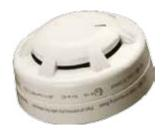
The Orbis I.S. Optical Smoke Detector works using the light scatter principle and is ideal for applications where slowburning or smouldering fires are likely.
