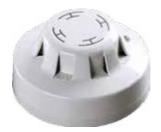
lonisation detectors use a low activity radioactive foil to detect fires by irradiating the air in the smoke chamber and causing a current flow. If smoke enters the chamber, the current flow is reduced leading to an alarm. Circuitry in the Integrating Ionisation Smoke Detector protects against transient levels of smoke above the normal threshold for up to 20 seconds.
