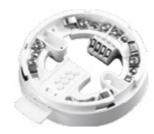
The Intelligent Heater Base is designed to be used in cold climates where environmental conditions could result in either icing or condensation affecting the operation of detectors. It is recommended that the heater base be used in conjunction with either a Waterproof Base Cover or Deckhead Mounting Box to minimise moisture ingress.
