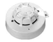
The Discovery Multisensor Detector comprises optical smoke and thermistor temperature sensors which give both a combined signal as well as a separate heat signal for improved false alarm management.
