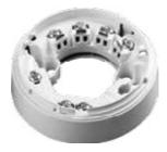
The Orbis Heater Base is designed to be used in cold climates where environmental conditions could result in either icing or condensation affecting the operation of detectors. It is recommended that the heater base be used in conjunction with either a Waterproof Base Cover or Deckhead Mounting Box to minimise moisture ingress.
