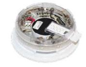
The XP95 Sounder VAD Base is a loop-powered sounder and EN 54-23 approved VAD combined with a standard intelligent mounting base. It is used to signal a fire alarm in enclosed areas.
