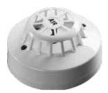
There are two heat detectors in the AlarmSense range designed to suit a wide variety of operating conditions. A static heat detector (CS) which responds only when a fixed temperature has been reached and a rate-of-rise detector (A1R) which has a fixed upper limit, but in addition, measures the rate of increase in temperature.
