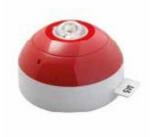
The Loop Powered VAD is designed for indoor use. The Category C VAD is specifically designed for use on a ceiling and comes in two different coverage classes. The two EN 54-23 coverage classes are C-3-8.5 and C-3 15. These devices are to supplement sounders in areas which carry the risk that sounders will not be heard.
