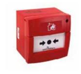
The XPander Manual Call Point is compliant with EN 54-11. It is wireless and is powered by two independent packs of three AA alkaline batteries with a typical five-year life.
