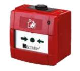
The Discovery Marine Manual Call Point has been approved for use in outdoor marine applications. A seven-segment DIL switch enables addressing of each call point at commissioning stage. When operated, the manual call point interrupts the polling cycle for a fast response. Bi-coloured LEDs indicate isolate and normal conditions.
