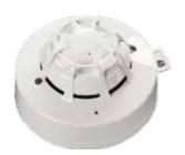
The XP95A Multisensor contains a photoelectric smoke sensor and a thermistor (temperature sensor) whose outputs are combined to give the final analogue value.
