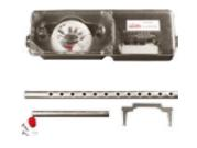
The Conventional Duct Smoke Detector provides early detection of smoke in the air moving through heating and ventilation (HVAC) ducts in commercial and industrial premises. Its purpose is to prevent the re-circulation of smoke from an area on fire to areas unaffected by the fire when used with a Series 65 or Orbis detector. It provides a volt-free changeover relay rated at 30V, 1A.
