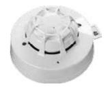
The XP95 Multisensor Detector contains an optical smoke sensor and a thermistor temperature sensor whose outputs are combined to give the final analogue value.
