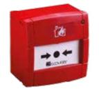
The Discovery Manual Call Point has a sevensegment DIL switch enables addressing of each call point at commissioning stage. When operated, the manual call point interrupts the polling cycle for a fast response. Bi-coloured LEDs indicate isolate and normal conditions.
