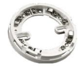
The Series 65 Standard Base has been designed to enable detectors to be fitted without the need of force – particularly useful when fitting to suspended ceilings. All Series 65 bases have a one-way only fit. Detectors can be locked into place by a grub screw using a 1.5mm hexagonal screwdriver.
