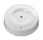
The Isolator is placed at intervals on the loop and ensures that, in the case of a short-circuit, only the section between the isolators will be affected. When the short-circuit is removed, the isolators automatically restore power and data to the isolated section.
