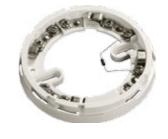
The Series 65 Diode Base is designed for use with conventional systems that have manual call points and detector bases on the same circuit. The base is fitted with a schottky diode on the 'L1 IN' and 'L1 OUT' wiring terminals. This base can only be used with compatible control equipment.
