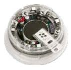
The XP95A Sounder Visual Indicator Base is a looppowered sounder and visual indicator combined with a standard Intelligent Mounting Base. It is used to signal a fire alarm in enclosed areas. The sounder visual indicator base can be used either with a detector fitted or with a cap for operation as a stand-alone alarm device.
