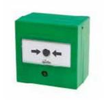
The Dual Switch Manual Call Point provides volt free double pole changeover contacts suitable for normally open or normally closed multiple switching from a single activation point. A device is activated by pressing the resettable element. An activation status is indicated through the rotation of the resettable element, displaying yellow and black indication bars. The manual call point can be easily reset from the front using the supplied reset key.
