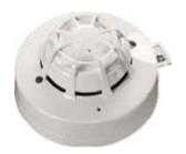
The Discovery UL Multisensor Detector consists of photoelectric smoke and thermistor temperature sensors whose outputs are combined to give the final analogue value. As a result, the multisensor is useful over a wide range of applications and is highly immune to false alarms.
