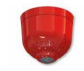
Sonos Pulse conventional ceiling mounted Visual Alarm Devices are available with a white and red flash colour. The white flash variant has an EN 54-23 approved coverage pattern of C-3-15, whereas the red flash variant has a coverage pattern of C-3-8.9.
