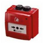
The Discovery Marine Waterproof Manual Call Point has been approved for use in outdoor marine applications. A sevensegment DIL switch enables addressing of each call point at commissioning stage. When operated, the manual call point interrupts the polling cycle for a fast response. Bi-coloured LEDs indicate isolate and normal conditions.
