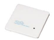
The XP95A Switch Monitor Input/ Output Module provides a voltagefree and single pole changeover relay output, a single, monitored switch input and an unmonitored, non-polarised opto-coupled input.
