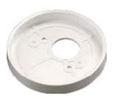
The Backplate provides a high degree of protection against the ingress of water or dust into the back of a detector mounted directly onto a mounting box. When the backplate is used with an XP95 device, the number tab of the XPERT card must be snapped off and placed in one of the knockout slots provided in the backplate.
