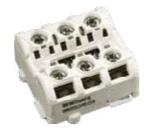
The Marine Mini Switch Monitor is an interface within an entirely new housing. Designed in response to customer feedback, the smaller Mini Switch Monitor can be fitted onto a 35mm DIN-Rail with a twist-click motion or mounted in an enclosure such as a manual call point. It is designed to monitor the state of one or more single pole, volt-free contacts connected to a single pair of cables and to report the status to Apollo-compatible control equipment.
