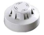
The AlarmSense Integrating Optical Smoke Detector works using the light scatter principle. The detector has the ability to monitor and discard transient sources of smoke.
