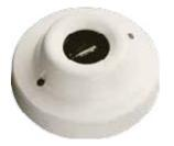
The Marine Intelligent Base Mounted UV IR<sup>2</sup> Flame Detector is designed to protect open indoor areas where open flaming fires may be expected. The detector has UV and dual IR sensors responding to different wavelengths to discriminate between flames and spurious sources of radiation.
