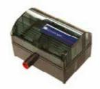
The Discovery Aspirating Smoke Detector (ASD) is a point based professional air-sampling unit, designed to complement analogue addressable system technology. It combines standard field serviceable smoke detectors with a stand-alone air sampling solution to provide protection of difficult to access, environmentally demanding, aesthetic or architecturally restricted areas.
