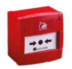
A seven-segment DIL switch enables addressing of each call point at commissioning stage. When operated, the manual call point interrupts the polling cycle for a fast response. Bi-coloured LEDs indicate isolate and normal conditions.
