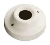
The Intelligent Base Mounted IR<sup>3</sup> Flame Detector is designed to protect all indoor areas, even in dirty or smoky conditions, where open flaming fires may be expected. The detector has three IR sensors that respond to different IR wavelengths in order to discriminate between flames and spurious sources of radiation.
