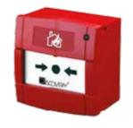
The Discovery Marine Manual Call Point has been approved for use in indoor marine applications. A seven-segment DIL switch enables addressing of each call point at commissioning stage. When operated, the manual call point interrupts the polling cycle for a fast response. Bi-coloured LEDs indicate isolate and normal conditions.
