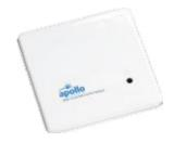
The XP95A 120V AC Input/Output module is a loop-powered device which incorporates a monitored input circuit for connection to dry contacts, in addition to a 120V AC 4A rated dry contact relay output. It is mounted in a plastic facia plate for use with a 4 square or two-gang electrical back box.
