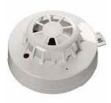
The XP95A Heat Detector monitors temperature by using a single thermistor which provides a voltage output proportional to the external air temperature. It is classified as an ordinary detector by UL.
