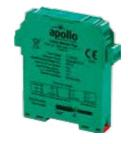
The DIN-Rail Switch Monitor Plus is designed to monitor the state of one or more single pole, volt-free contacts connected on a single pair of cables and to report this status to Apollo-compatible analogue addressable control equipment.
