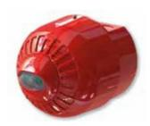
Sonos Pulse conventional wall mounted Visual Alarm Devices are available with a white and red flash colour. The white flash variant has an EN 54-23 approved coverage pattern of W-3.1-11.3, whereas the red flash variant has a coverage pattern of W-2.4-7.5.
