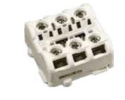
The Mini Monitor Module is an interface within an entirely new housing. This allows the unit to be fitted onto a standard 35mm DIN-Rail (using a twistclick motion) or mounted within an enclosure, for example a Pull Station. It is designed to monitor the state of one or more single pole, voltage-free contacts connected on a single pair of cables and to report this status to Apollocompatible analogue control equipment.
