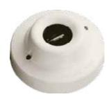
The Conventional Base Mounted UV Flame Detector is designed to protect enclosed indoor areas where open flaming fires may be expected. The detector has a fast-acting response to flames up to 25m away and is equipped with a single UV sensor with a narrow spectral response in order to discriminate between flames and most spurious sources of radiation.
