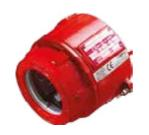
The Intelligent Flameproof IR<sup>3</sup> Flame Detector is designed for hazardous environments in either indoor or outdoor applications. It is sensitive to low-frequency, flickering infra-red radiation emitted by flames during combustion. These detectors are BASEEFA approved and meet the requirements of ATEX Directive 94/9/EC.
